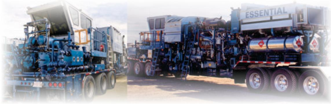
ECWS fluid pumping equipment is designed to meet the requirements of the toughest wellbore(s). The pumpers perform such duties as coil assist, wireline pumpdown, diagnostic fracture injection test (DFIT), and various high horsepower applications. ECWS fluid pumpers provide a full range of coiled assist abilities that provide an economic advantage and the ability to transport both surface iron and treatment chemicals.
