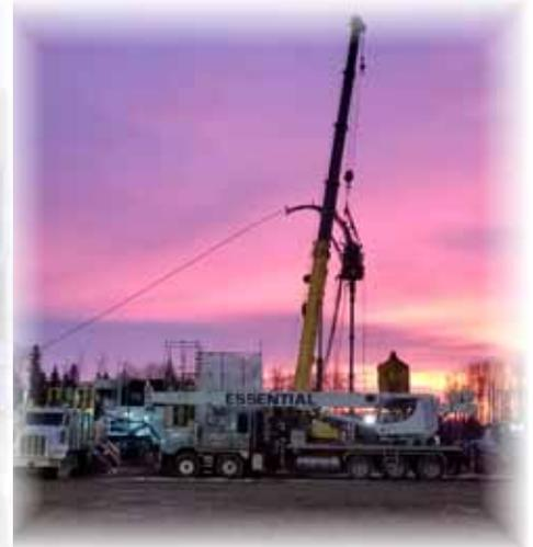
Generation I coiled tubing units offer versatility for a wide range of specialty applications utilizing smaller pipe diameters and unique wellhead configurations. Our Gen I's operate coil sizes ranging from 38.1 mm (1.500 in) to 60.3 mm (2.375 in) with a reel capacity to reach customer's desired total depth.
