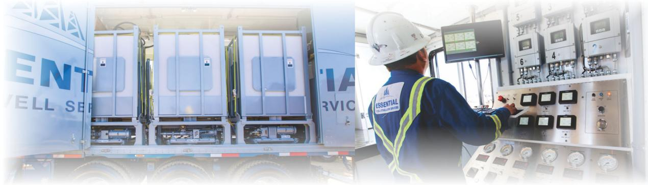
ECWS chemical vans have six fluid injection pumps and six 1,000 L totes. Our chemical trailers are outfitted with eight fluid injection pumps and ten 1,000 L totes in a large format tractor-trailer unit. The pumps in both units have low and high rate ability; all chemical totes are temperature controlled for any weather conditions.
